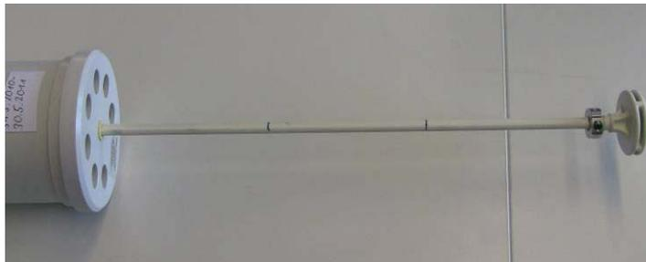
Attach the EasyOne Pro flow sensor tightly to the 3L calibration syringe using the special ndd calibration adapter. Make sure that the flow path is properly aligned.
