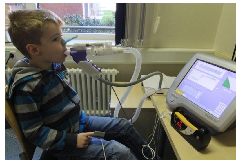
Figures 3 and 4: MBW N2b with EasyOne Pro LAB™ and corresponding screenshot with real time traces of flow and molar mass and automated analysis
